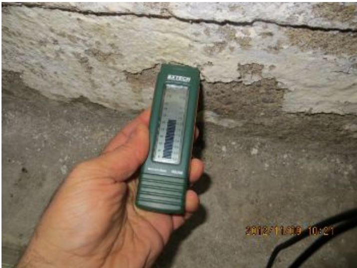
Active leaks observed at the time of inspection.
